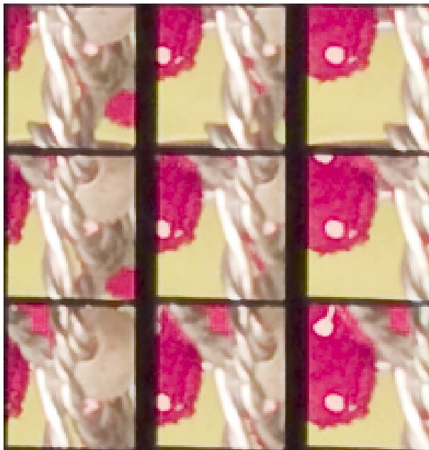
Figure 2: A crop of a raw lightfield capture. Each of the nine smaller images are referred to as a microimage.
